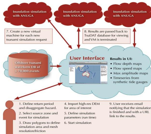
**Figure 1: The TsuDAT architecture and workflow**
